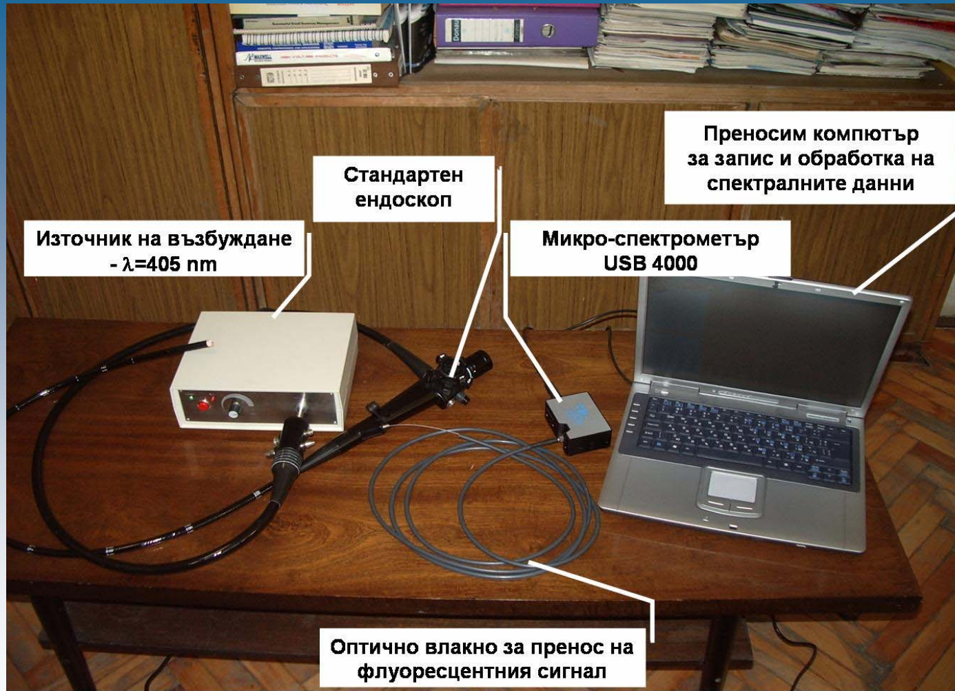
Optical system for fluorescence spectroscopy of the gastrointestinal tract
